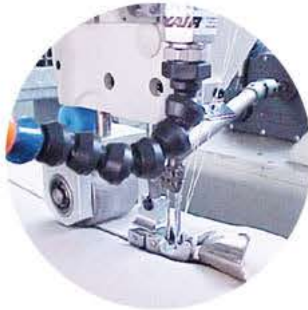
Thermo welded Seam
